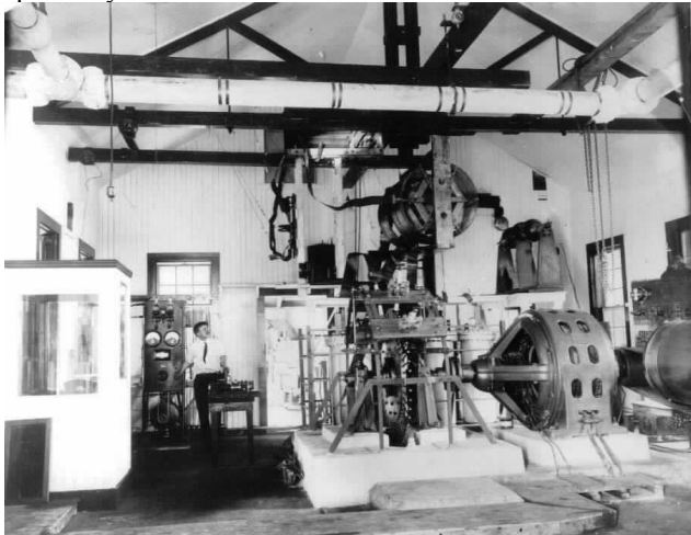
Figure 3 Fessenden's synchronous spark gap transmitter, Brant Rock, MA. The operator is Guy Hill (credit National Museum of American History, Smithsonian Institution, Washington, DC).
