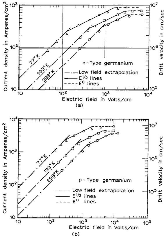
Fig. 4. (a, b). Current density as a function of electric field.
