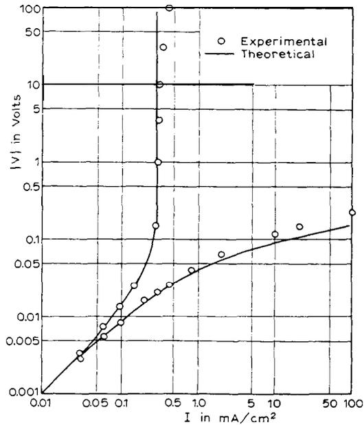
Fig. 9. Rectification characteristic for a p-n junction.
