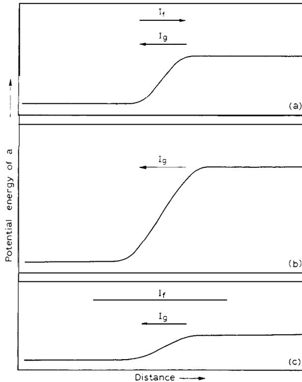
Fig. 8. Dependence of recombination and generation currents upon bias. (a) Thermal equilibrium; (b) reverse bias; (c) forward bias.
