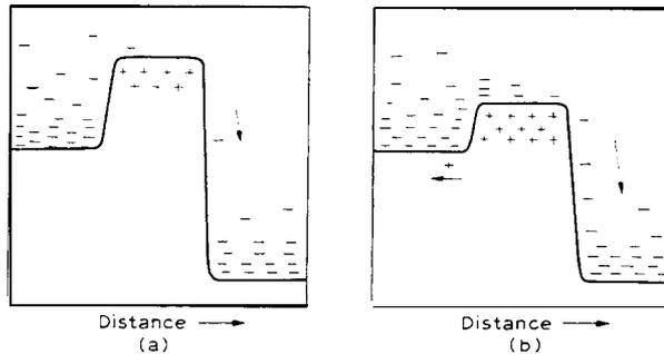
Fig. 12. The potential energy of an electron in an n-p-n junction transistor for two values of bias across the emitter junction. In (b) the forward bias is greater than in (a).
