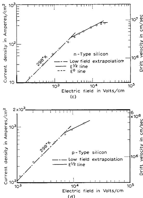
Fig. 4. (c, d). Current density as a function of electric field. (c) n-type silicon; (d) p-type silicon.
