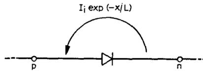
Fig. 10. Equivalent circuit for a p-n junction photocell.
